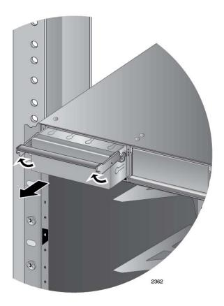
Figure 56. Removing the Blank Slot Cover from Power Supply Slot A
